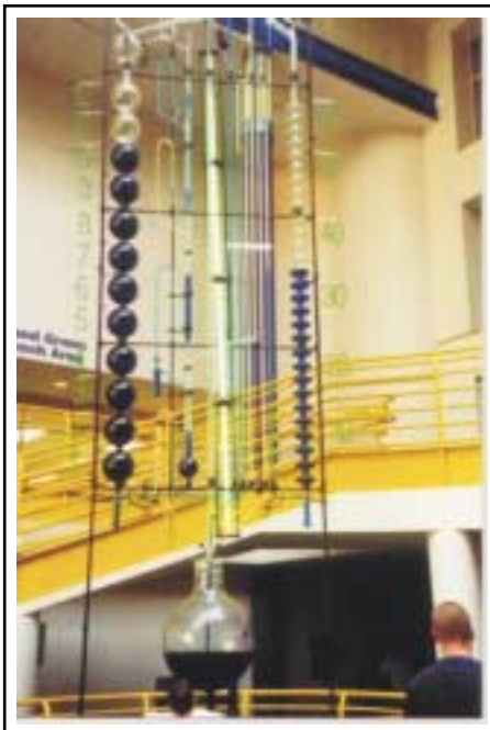
The Indianapolis Children's Museum water clock. Hour spheres on the left, 2-minute disks on the right. The time is now ... 10:32.
